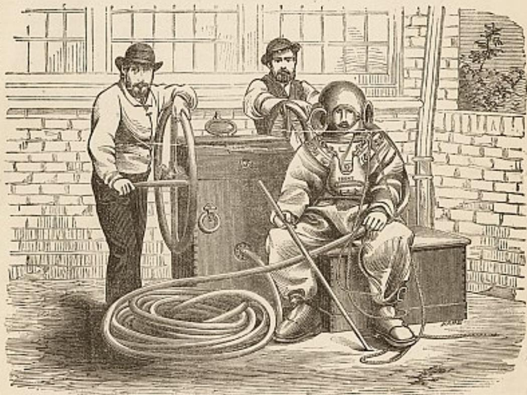
The front Eye of Helmet is shown open, and is not closed till just previous to the Diver descending into the water.
