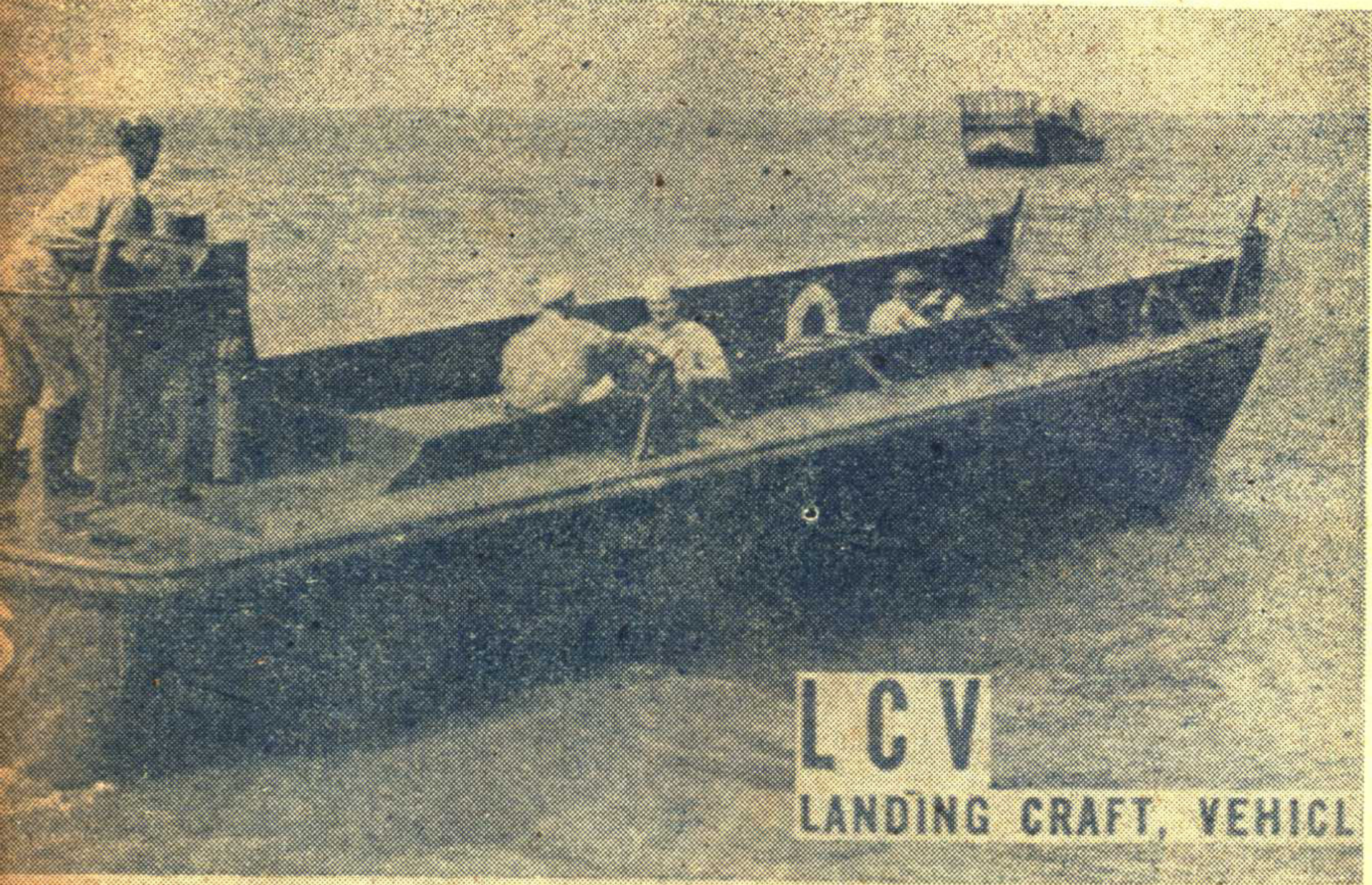
LCV, similar to LCVP, is used for landing troops and light vehicles. It is 96 feet long, has a medium speed motor and mounts machine guns. The ramp and sides are armored.
