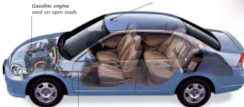
Electric motor and generator used in cities
