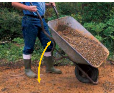
◀ WHEELBARROW A wheelbarrow is free to pivot around the large wheel at the front. When the worker lifts the handles, the force causes the entire wheelbarrow to swing upward and turn around the wheel. The long body and handles of a wheelbarrow increase the turning effect and make it easier to dump out a heavy load.
