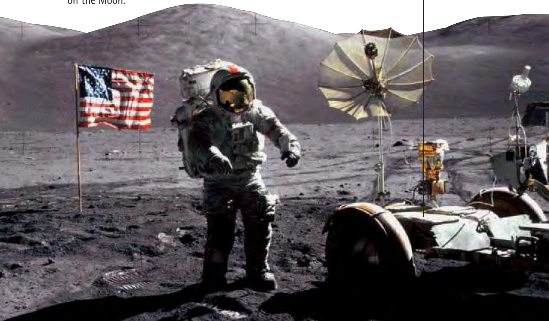
Lunar rover, powered by electric motors, has a top speed of 10 mph (16 kph).
