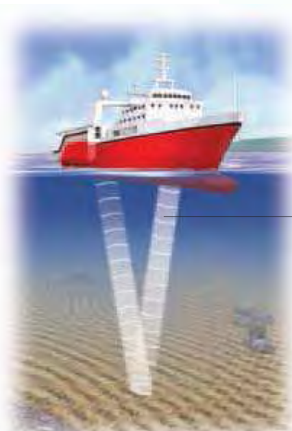
Ultrasound waves are sent to the seabed and echo back to the ship
