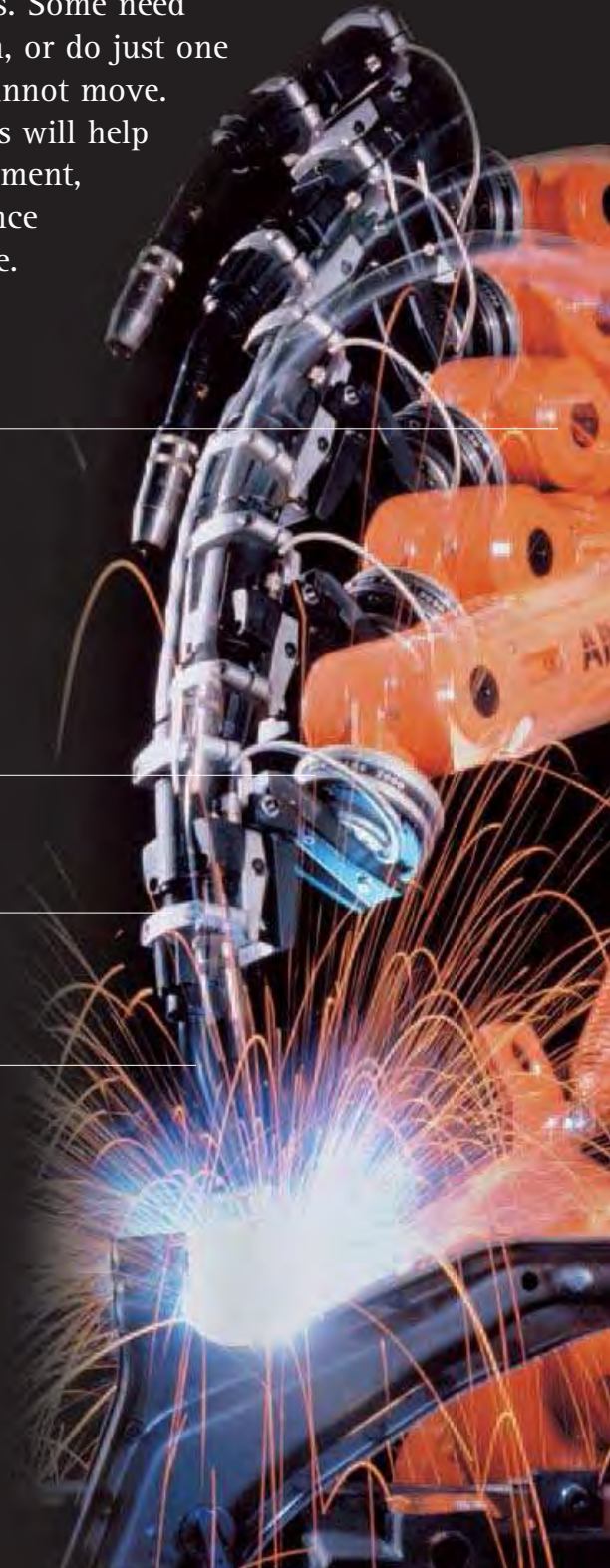
Arm can pivot up and down and extend telescopically in and out
