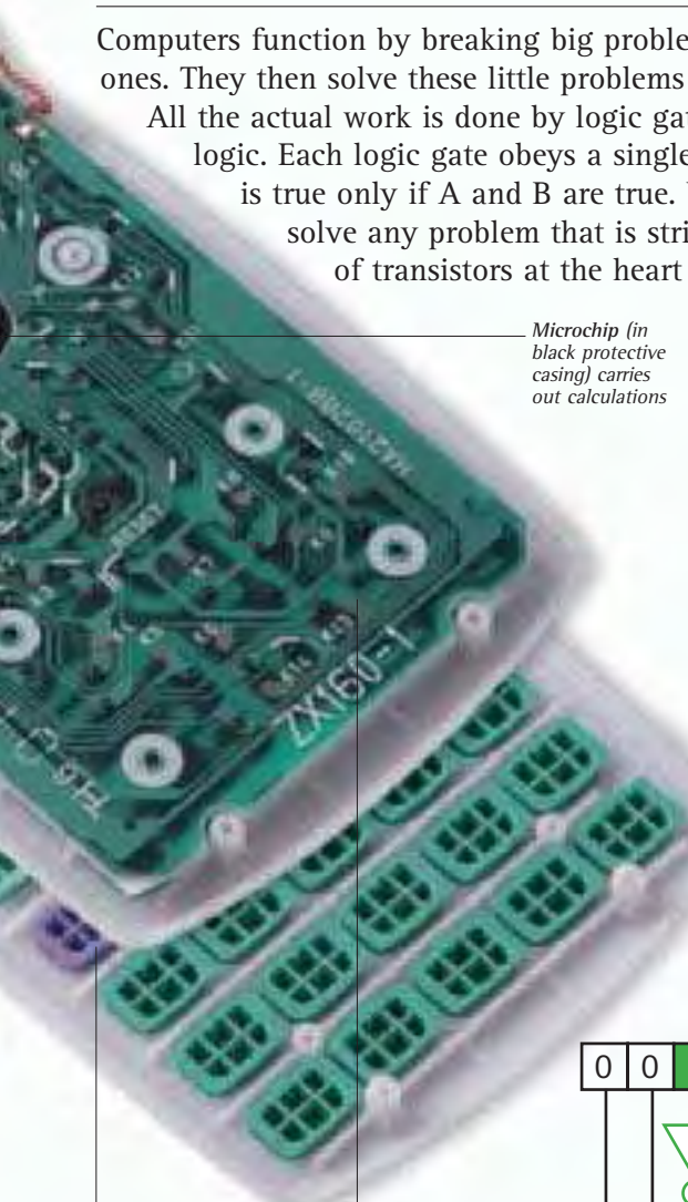
Keys operate contacts on the circuit board
