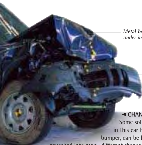
Plastic bumper bends and changes shape
