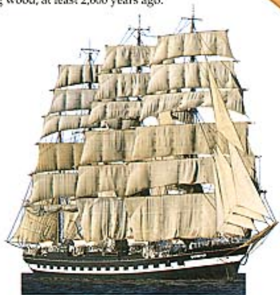
WHAT IS A SHIP? All large vessels are usually called ships, but this word also has a precise meaning. A ship has three or more masts all rigged with square sails. The Kruzenshtern's fourth mast has fore-and-aft sails (pp. 24–25), which makes her a "barque", not a ship.
