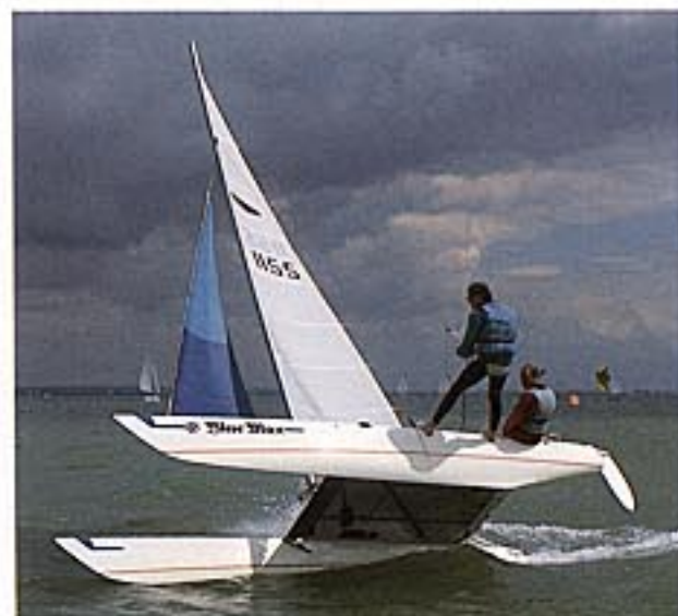
DARTING ABOUT The dart is a catamaran, a twin hulled boat (p. 60). Because these boats are so wide, they can carry a lot of sail, so they are very fast and make for exciting sailing. The dart has no centreboard or boom, which keeps the cost down.
