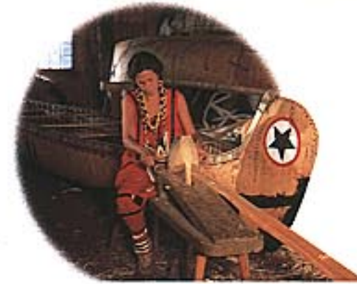
STIFFENING A canoe can be made with no more than an axe and a knife. This woman is carving a rib from a piece of spruce. It will be lashed on the inside to stiffen the canoe's bark shell.
