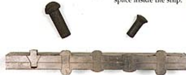
METAL PEGS These are some of the types of rivets used in shipbuilding to fasten overlapping iron or steel plates together.
