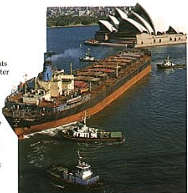
BULKY CARRIER Like most modern ships, this "bulk carrier" is too big and cumbersome to manoeuvre in a harbour under its own steam. Instead she (all ships are usually called "she") is being pushed and pulled by tugs. Some bulk carriers can carry over 200,000 tonnes of cargo. But they are small compared to most oil tankers, which can carry twice as much.
