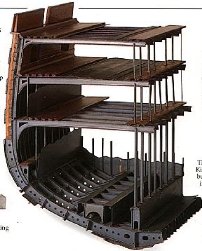
Metal bulkheads, which divide a ship into watertight compartments, have just been added to this steamer
