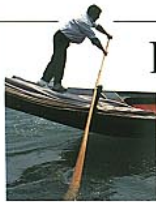
CROOKED CONSTRUCTION The gondola is fatter and wider on one side, the port side, than the other. This means the gondolier can row with one oar and still go in a straight line.
