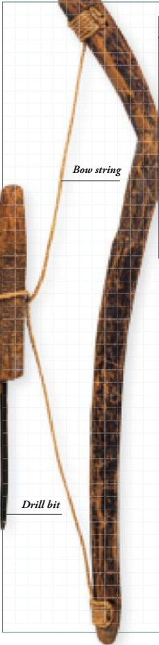
Bow drill Drilling was done using a bow, which was wrapped around the drill handle and moved back and forth to turn the drill fast enough to bore holes in wood or stone. Materials Copper (drill bit), wood (handle), string Uses Drilling holes Amazing fact The Egyptians could even drill holes in hard stones, such as granite, by using sand with broad copper drills.
