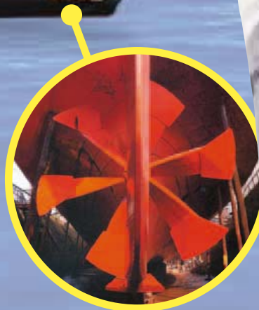
SS Great Britain had a six-blade propeller. Previous ocean-going ships had side paddle wheels.
