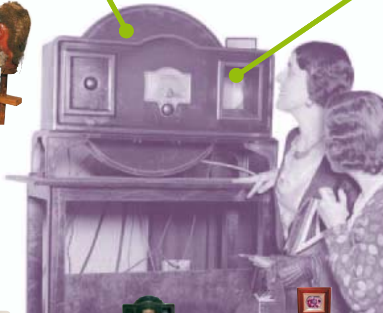
Baird used a spinning Nipkow disc in his televisor.
