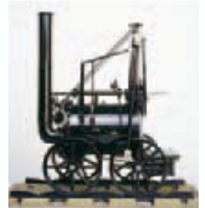
Steam travels along this pipe to the pistons.
