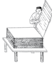
Pressing the screen to remove the water
