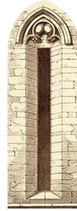
SLIT WINDOW Because glass was expensive, early medieval windows were often just a simple slit in the wall. Sometimes the window had a flat top, sometimes a pointed head, called a lancet.
