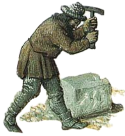
Dressing a stone block with an axe
