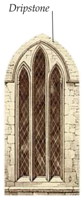
THREE IN A ROW By about 1230, lancets were often arranged together in groups to form a window. Each lancet is called a "light," so this is a "three-light" window. Rain is diverted by the dripstone above.
