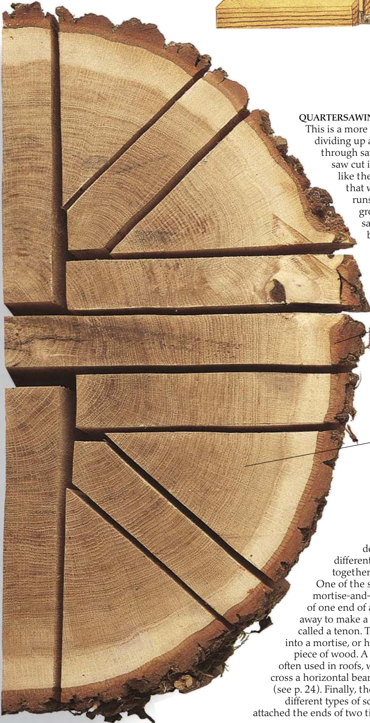
Radial boards are cut at right angles to the grain
