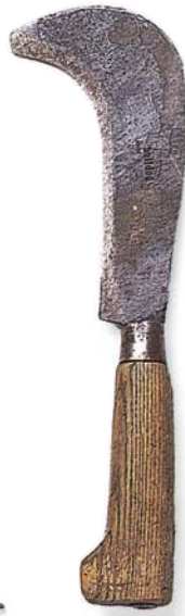
Spar hook, to shave spars and rods
