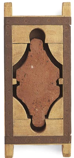
Mullion brick in its wooden mold
