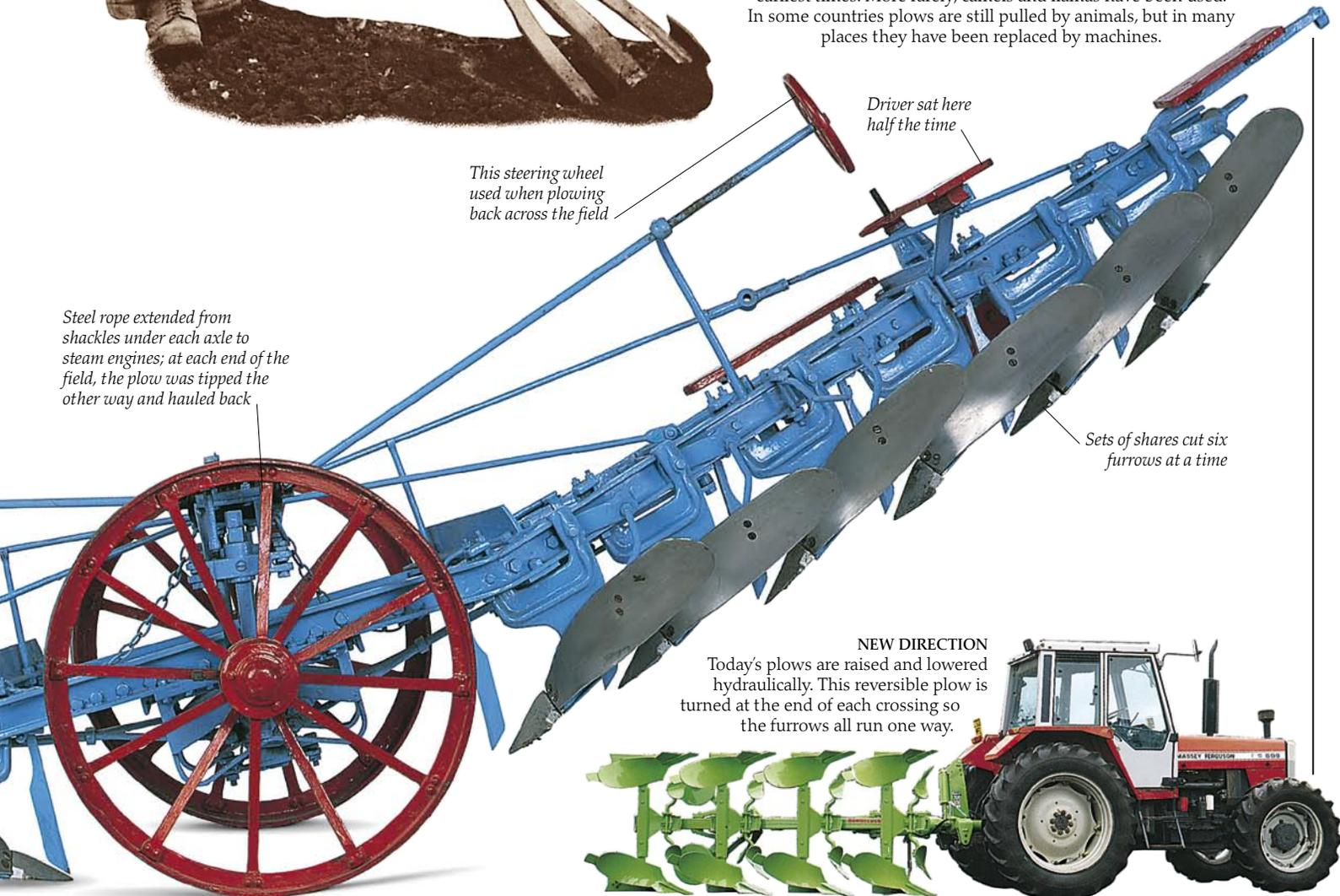
Steel rope extended from shackles under each axle to steam engines; at each end of the field, the plow was tipped the other way and hauled back
