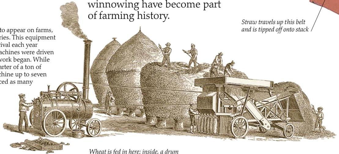
Straw travels up this belt and is tipped off onto stack
