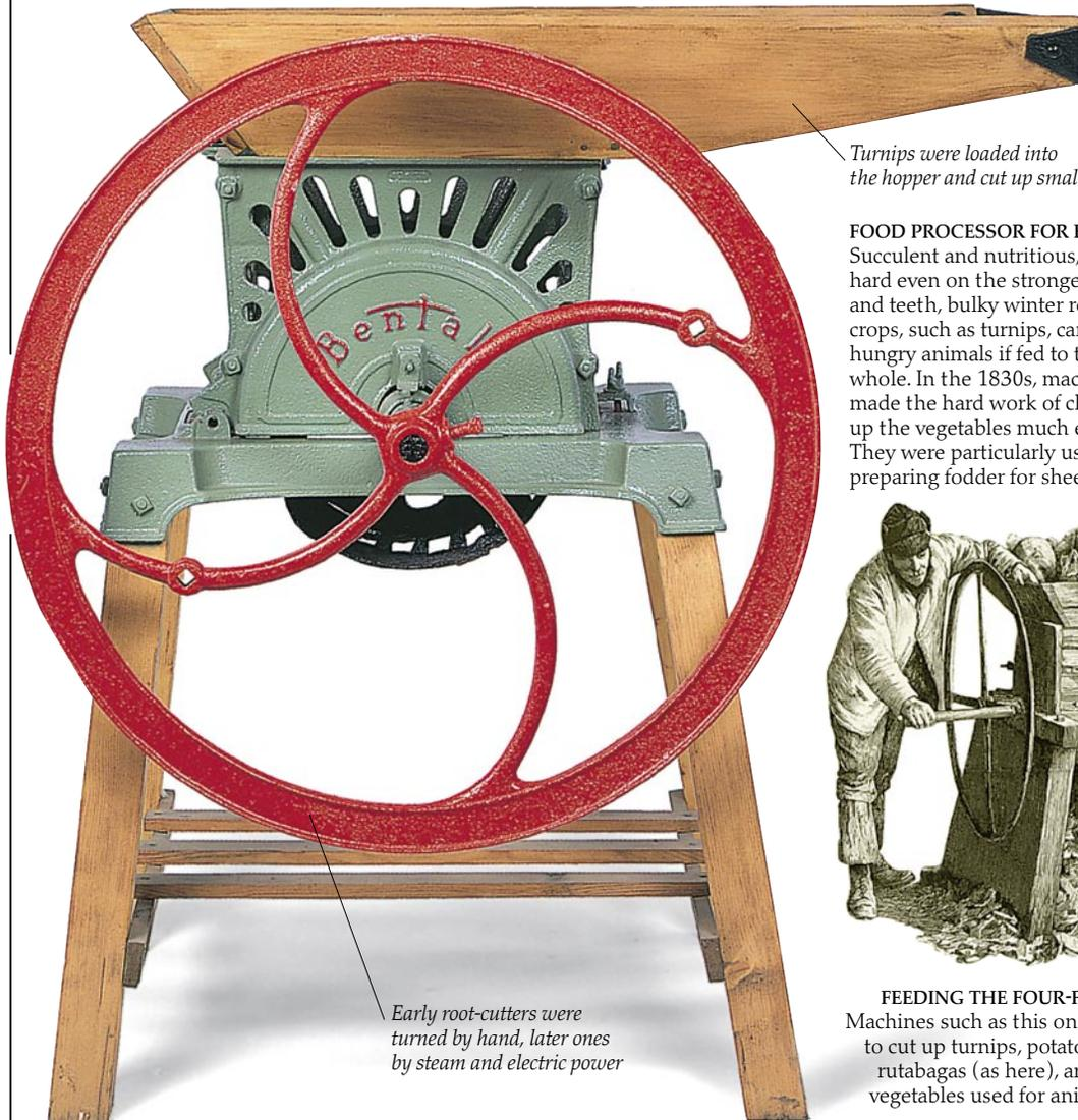
Turnips were loaded into the hopper and cut up small
