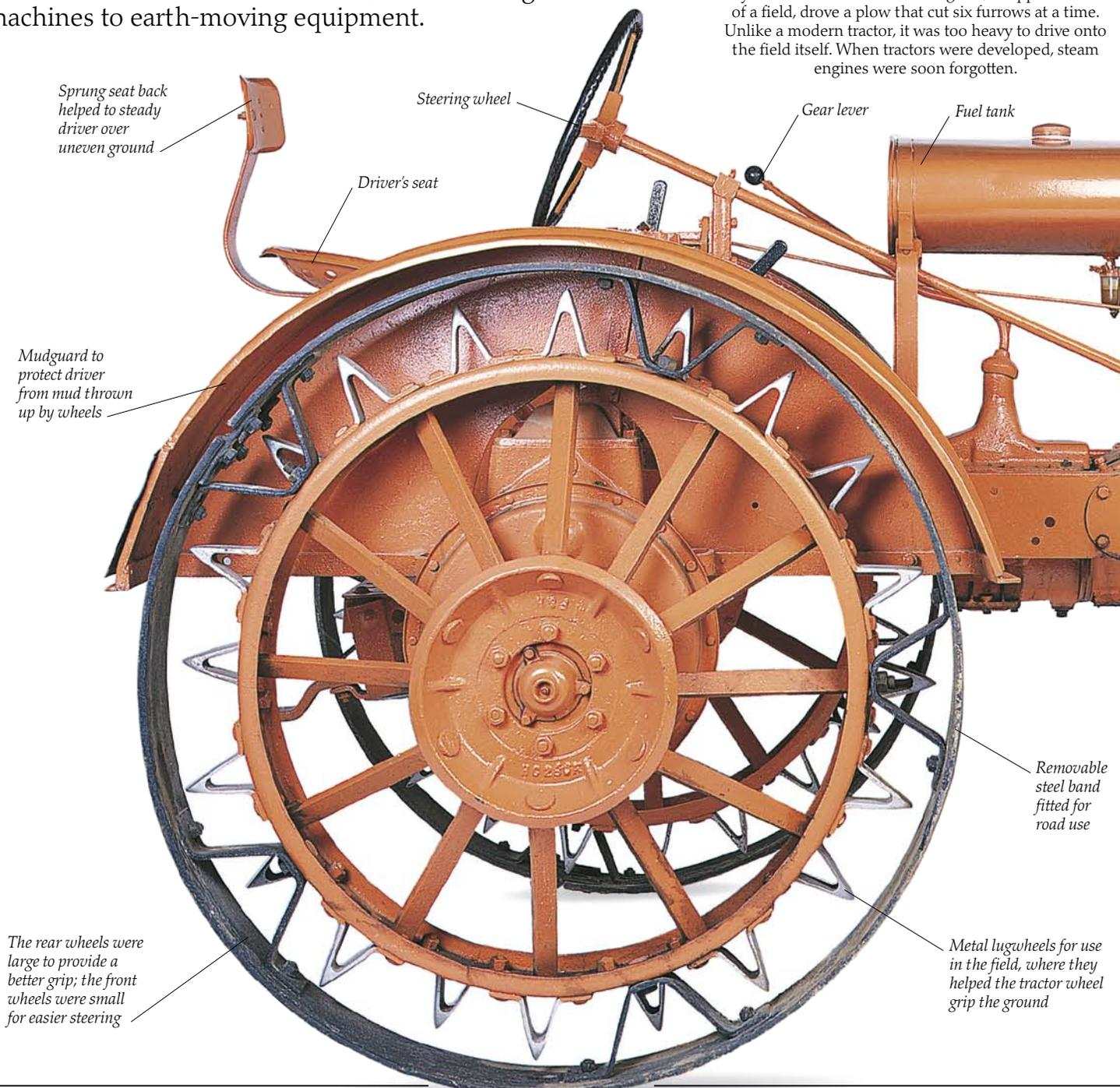
*Sprung seat back helped to steady driver over uneven ground*
