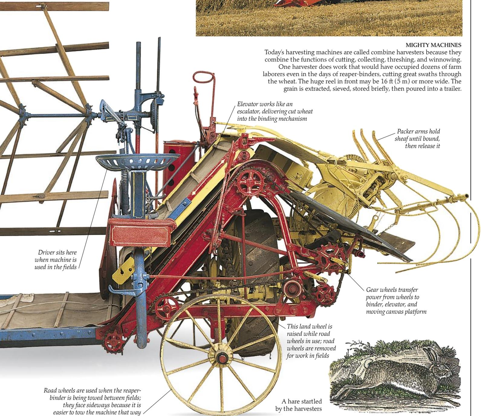
Elevator works like an escalator, delivering cut wheat into the binding mechanism
