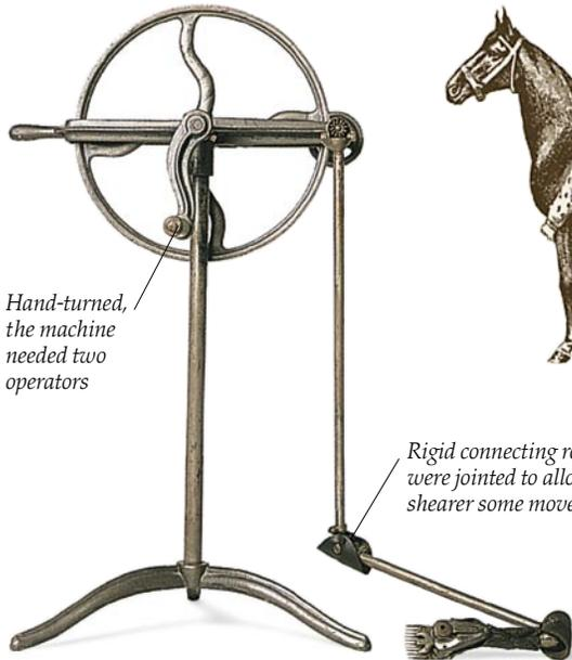
Hand-turned, the machine needed two operators
