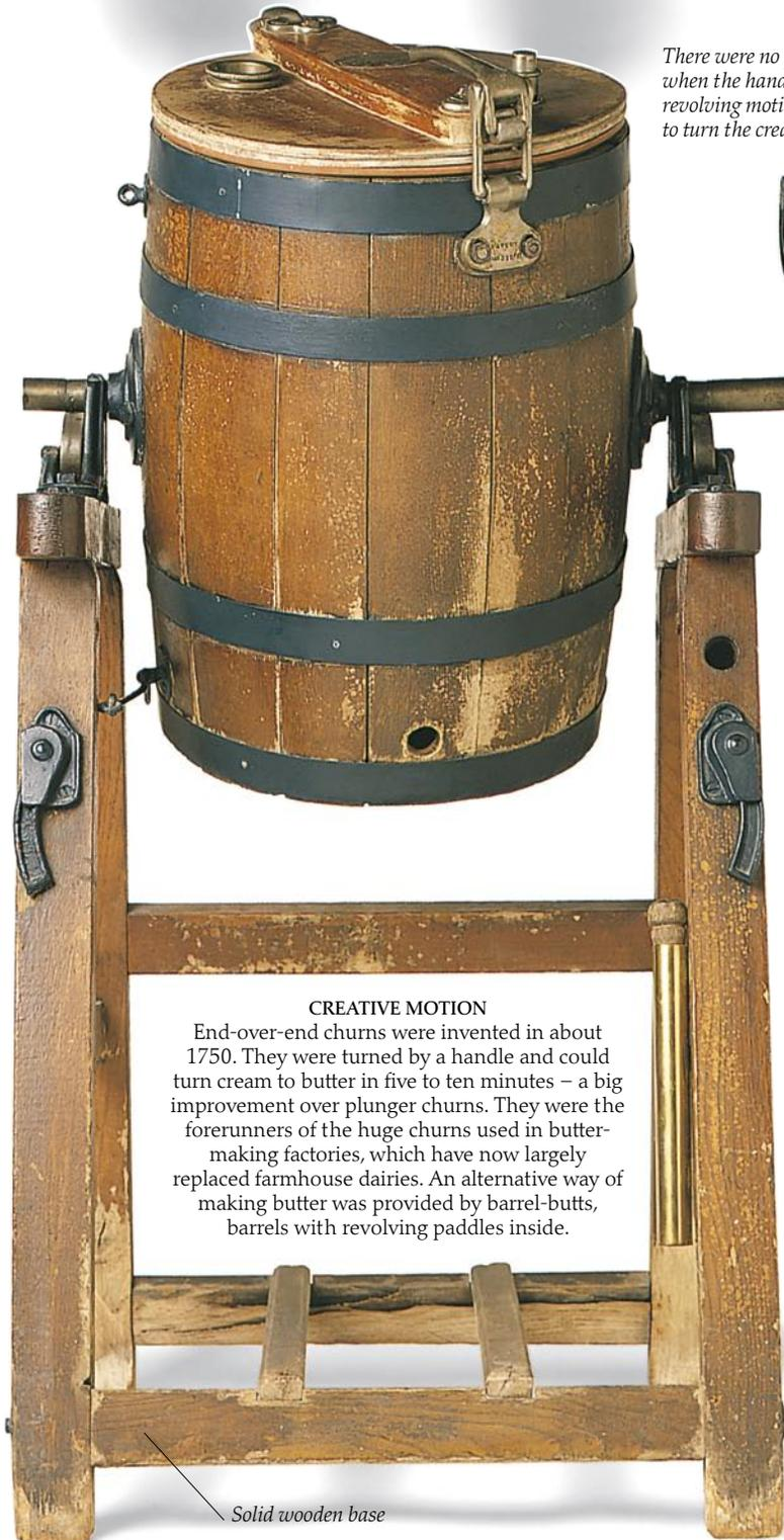
*There were no paddles inside; when the handle was turned, the revolving motion was enough to turn the cream into butter*
