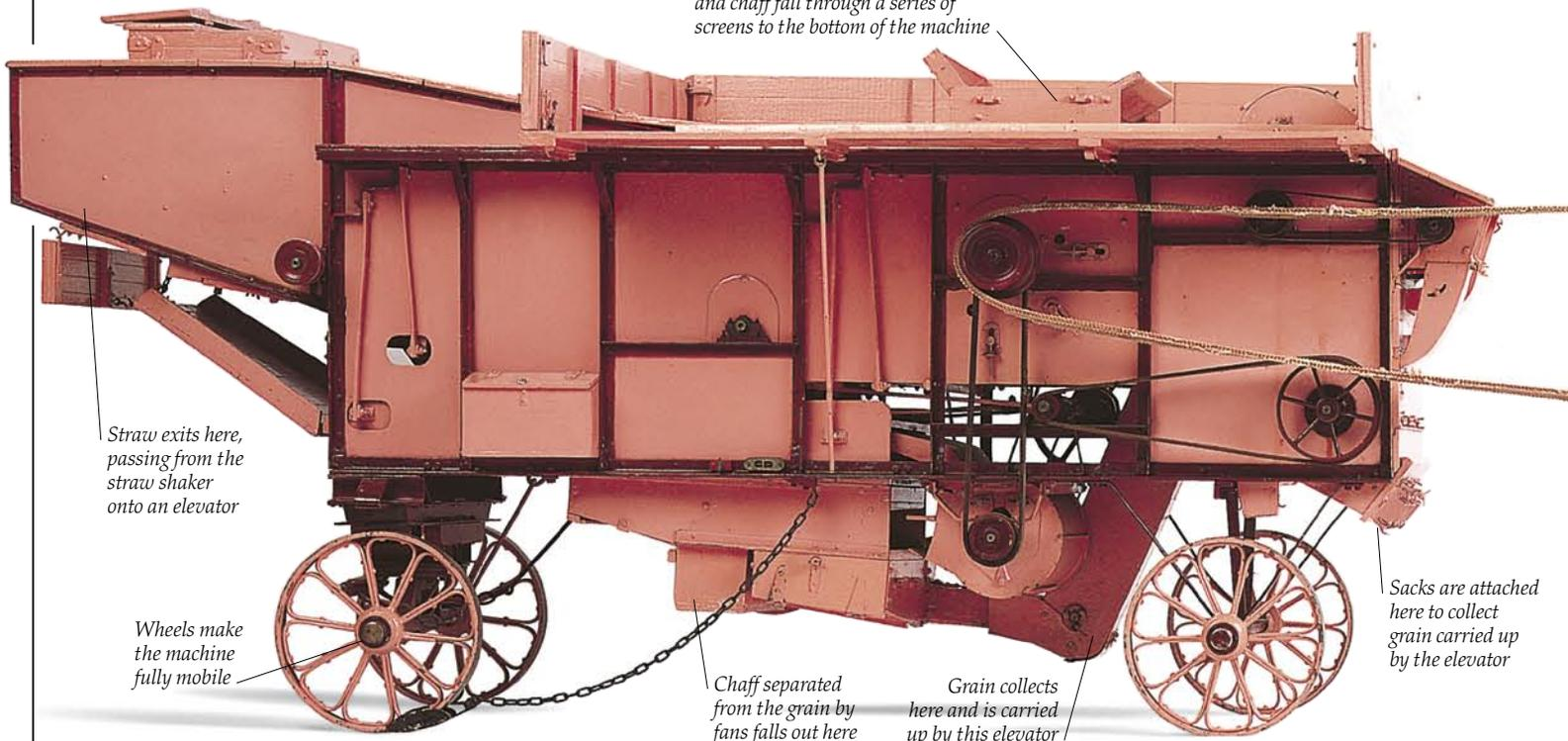
Straw exits here, passing from the straw shaker onto an elevator
