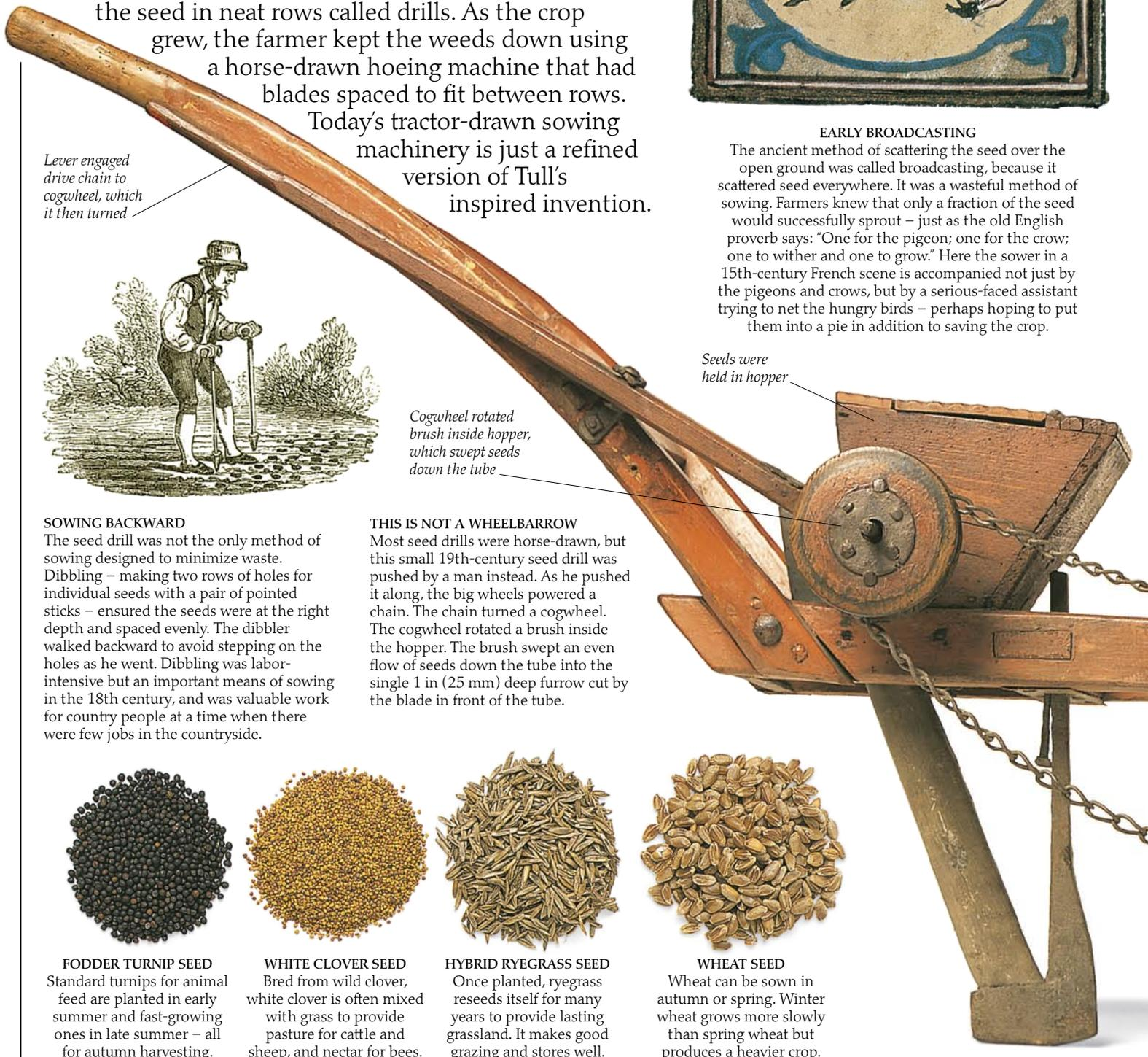
Lever engaged drive chain to cogwheel, which it then turned
