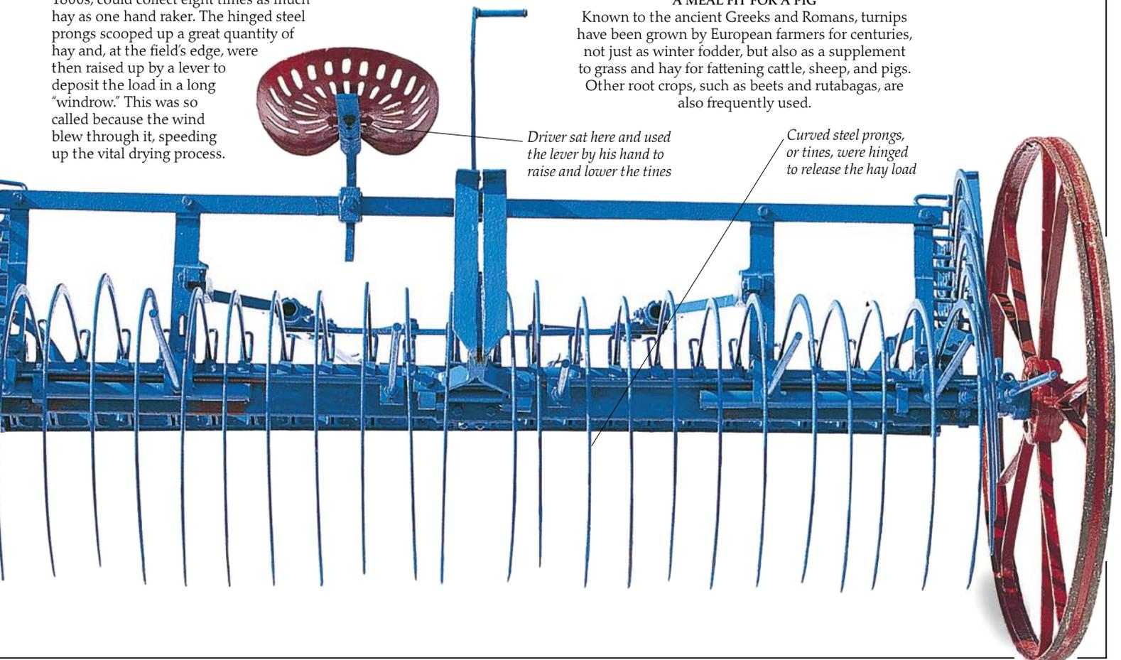
*Driver sat here and used the lever by his hand to raise and lower the tines*
