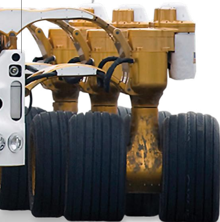
Platform lowers to ground for loading and stepping on and off
