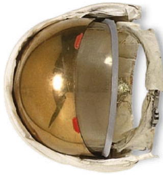
Outer helmet worn on the Moon has adjustable Sun shields and visors
