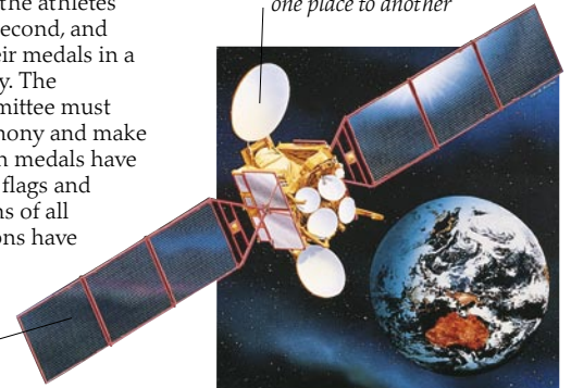
Dish reflects radio signals from one place to another
