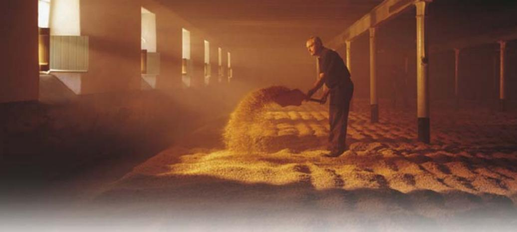
**On a traditional maltings floor**, such as this one at Balvenie, the grain is turned by hand to aerate it and so promote an even rate of germination.
