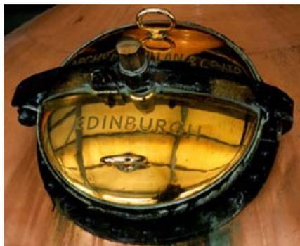
“Man doors” are a feature of pot stills. They can be opened up to inspect and clean the insides between distillation batches.
