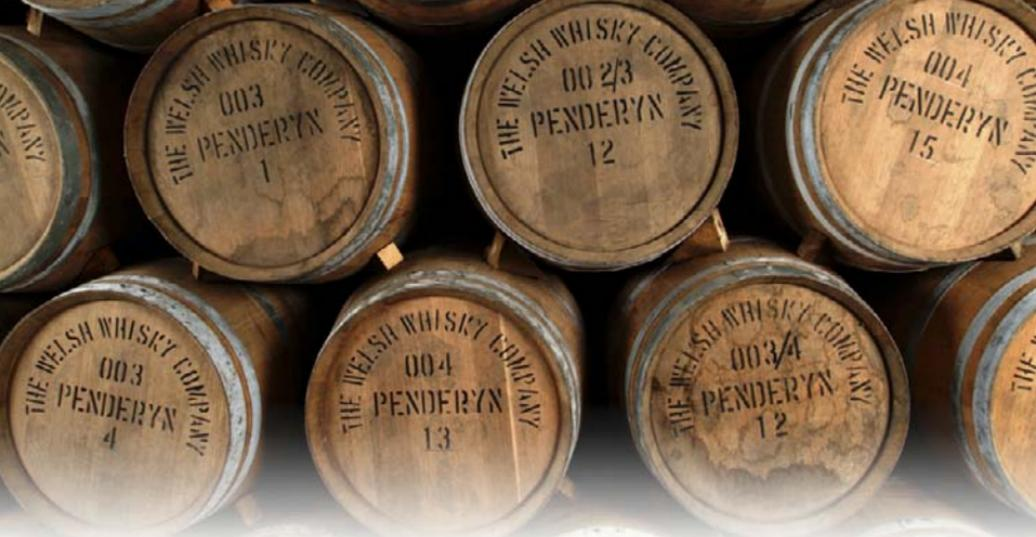
Bourbon is matured in barrels (which hold around 44 gallons, or 200 liters). Some are shipped from the US intact as “American Standard Barrels,” but most are broken down into their staves and arrive in bundles called shooks. In Scotland they are reassembled in a slightly larger, 55-gallon (250-liter) format called a re-made hogshead.
