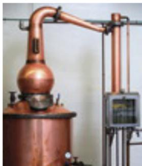
**At Bakery Hill** the spirit is distilled in a copper pot still and passed through a locked spirit safe.
