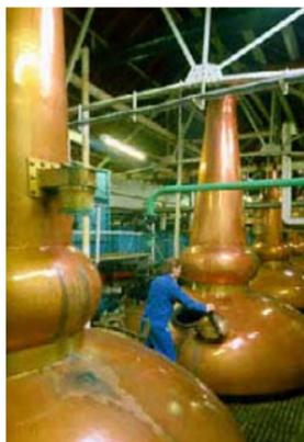
**As with most Scotch whiskies,** the wash at Tomatin is distilled twice in copper pot stills.
