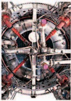
Nozzle where gases produced by burning fuel in the booster rocket are expelled
