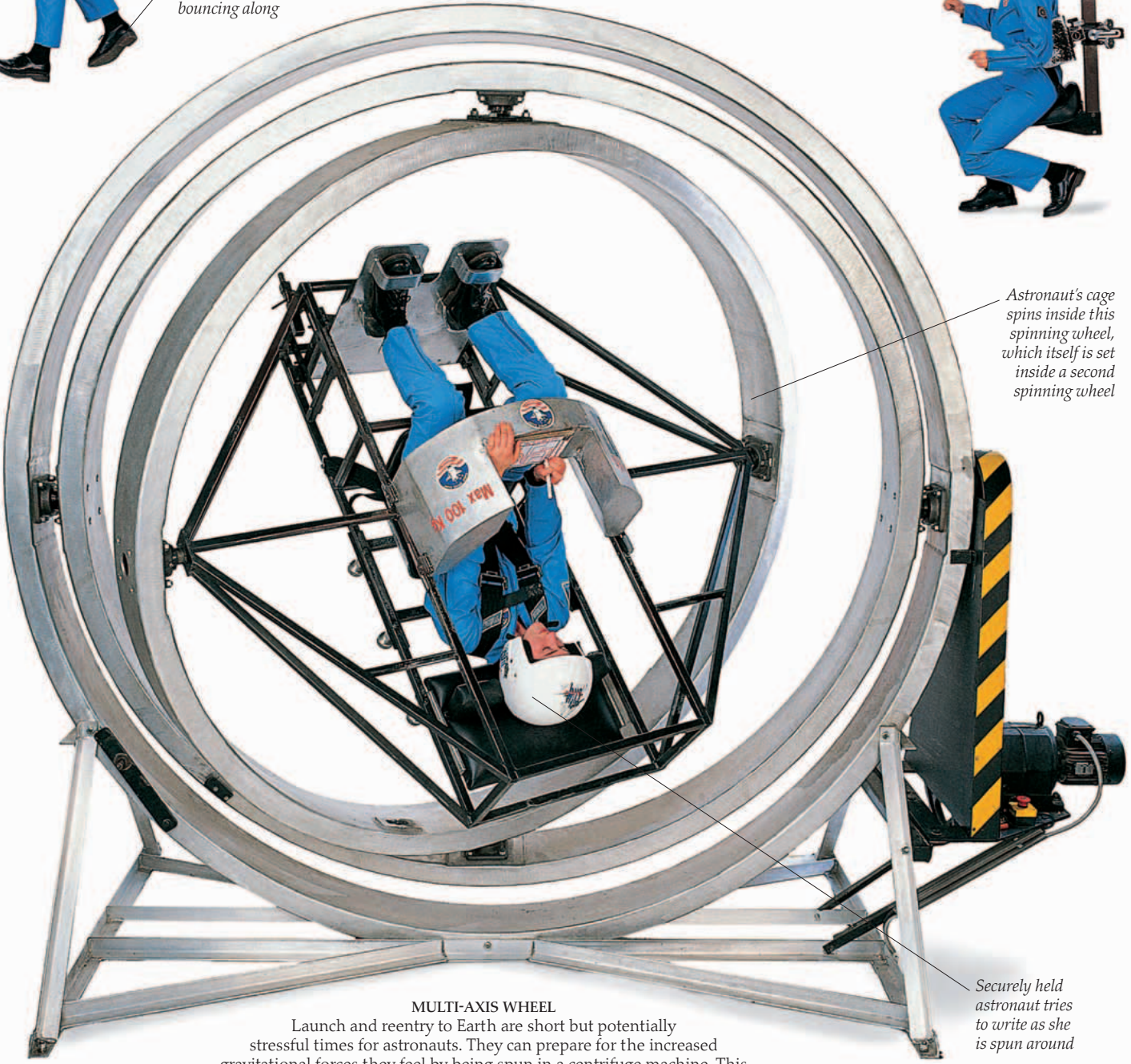
Back harness helps to keep the astronaut upright
