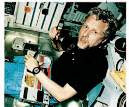
Food packages held on a tray, which is strapped to the astronaut's leg
