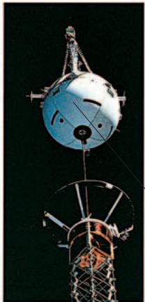
With only about 30 ft (10 m) to go, the tether broke and the satellite was lost
