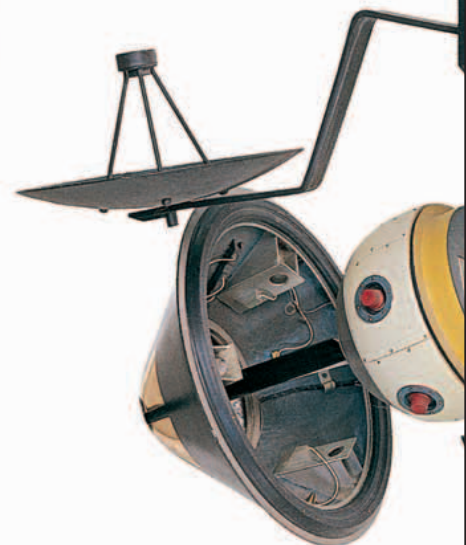
Boom with magnetometer to measure magnetic field in interplanetary space and near Jupiter
