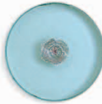
Potential damage of space dust on shuttle window
