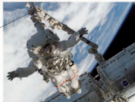
Arm has seven motorized joints
