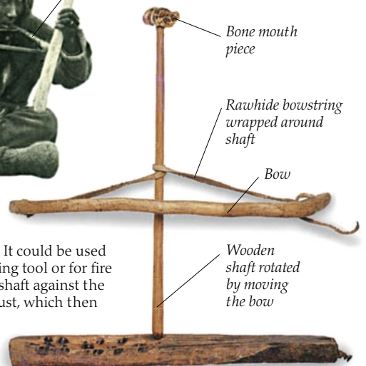
Bow drill used to carve ivory cribbage board, c. 1902
