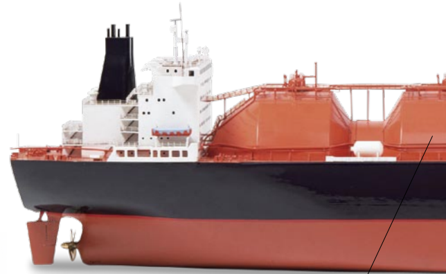
A typical LNG tanker holds more than 40 million gallons (150 million liters) of LNG, with an energy content equivalent to 24 billion gallons (91 billion liters) of the gaseous form
