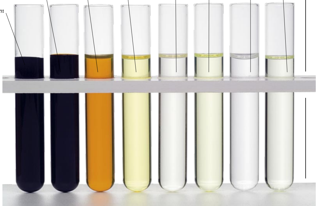
Fuel oil (for power plants and ships) Heavy lubricating oil Medium lubricating oil Light lubricating oil Diesel Jet fuel (kerosene) Gas
