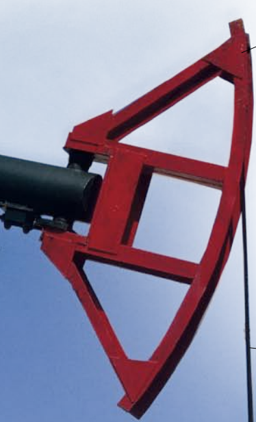
The curved end of the beam is likened to a donkey's head
