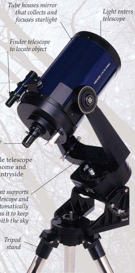
Finder telescope to locate object
