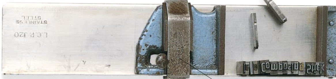
Adjustable grip to set width of lines
