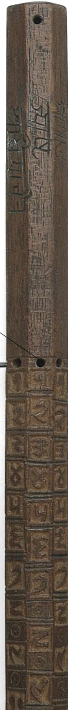
TIBETAN TIMESTICK The Tibetan timestick relied on the shadow cast by a pin through an upright rod. The pin would be placed in different positions according to the time of the year.
