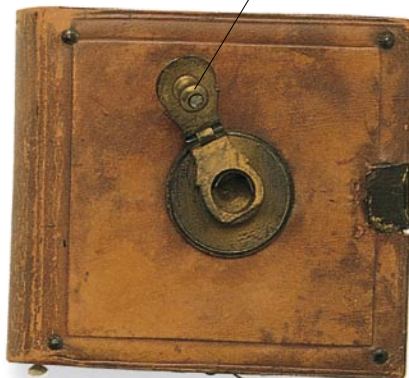
Winder to take up tape into container
