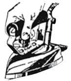
ELECTRIC IRON The first electric iron was heated by an electric arc between carbon rods and was highly dangerous. A safer iron was patented in 1882. It used an electrically heated wire element like the coils on a stove.
