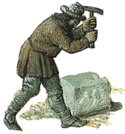
Dressing a stone block with an axe
