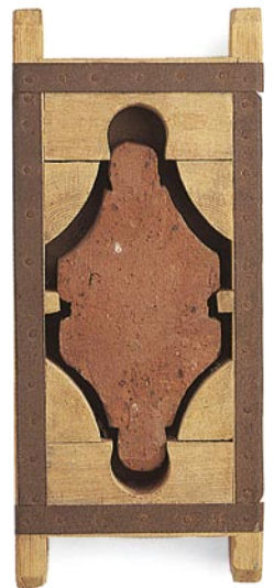
Mullion brick in its wooden mold
