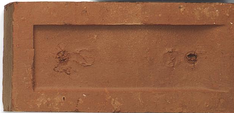
BRICKS Easily moulded clays are fired to make bricks. Impurities in clays produce bricks of different colours and strengths, making them suitable for a variety of uses.
