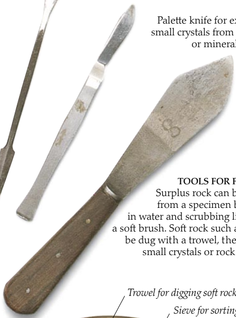
Spatulas for fine work, such as cutting around fossils
