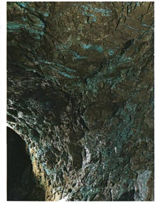
Section of a mine roof colored with deposits of the copper mineral, chalcantite
