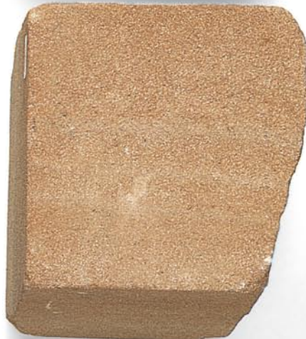
Red sandstone from Scotland used as a cladding building stone
