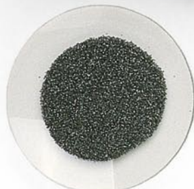
Coarse grinding grit used in first tumbling
