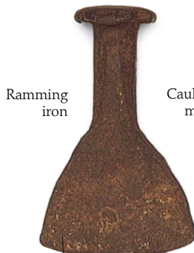
Broad blade for splitting open rotten seams
