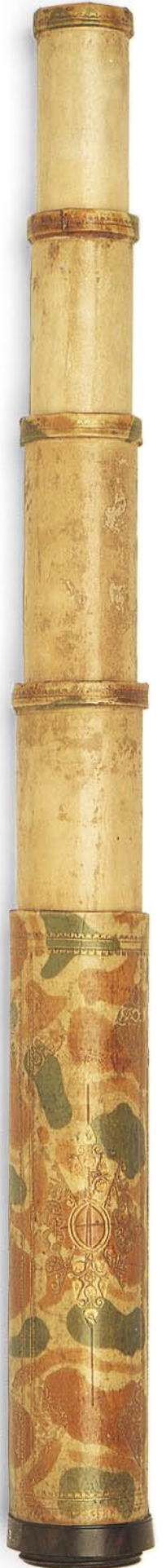
Late-17th-century telescope with tube of paper and vellum
