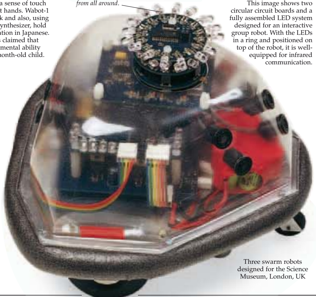
The LEDs form a circle so their light can be detected from all around.
