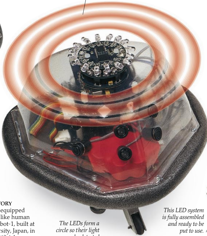
The rubbery bumper contains bump sensors.
