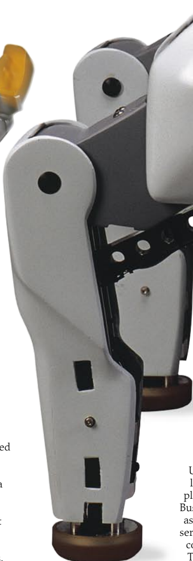
GUARD DRAGON Banryu, whose name means "guard dragon," can walk at 50 ft (15 m) a minute and step over a 6-in (15-cm) threshold. It can smell burning, see, and hear. If Banryu detects danger, it reports by cell phone to its owner, who can control it remotely.
