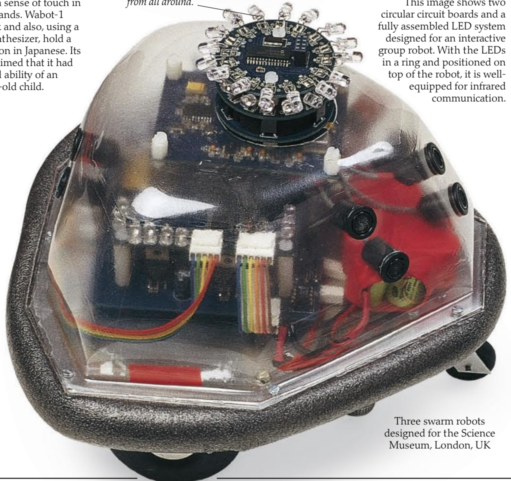
The LEDs form a circle so their light can be detected from all around.
