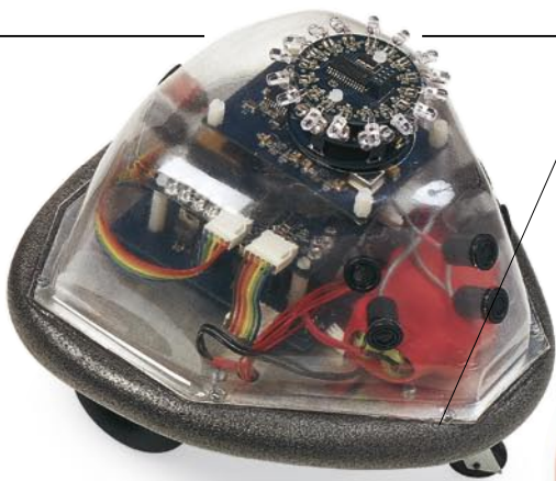
The rubbery bumper contains bump sensors.
