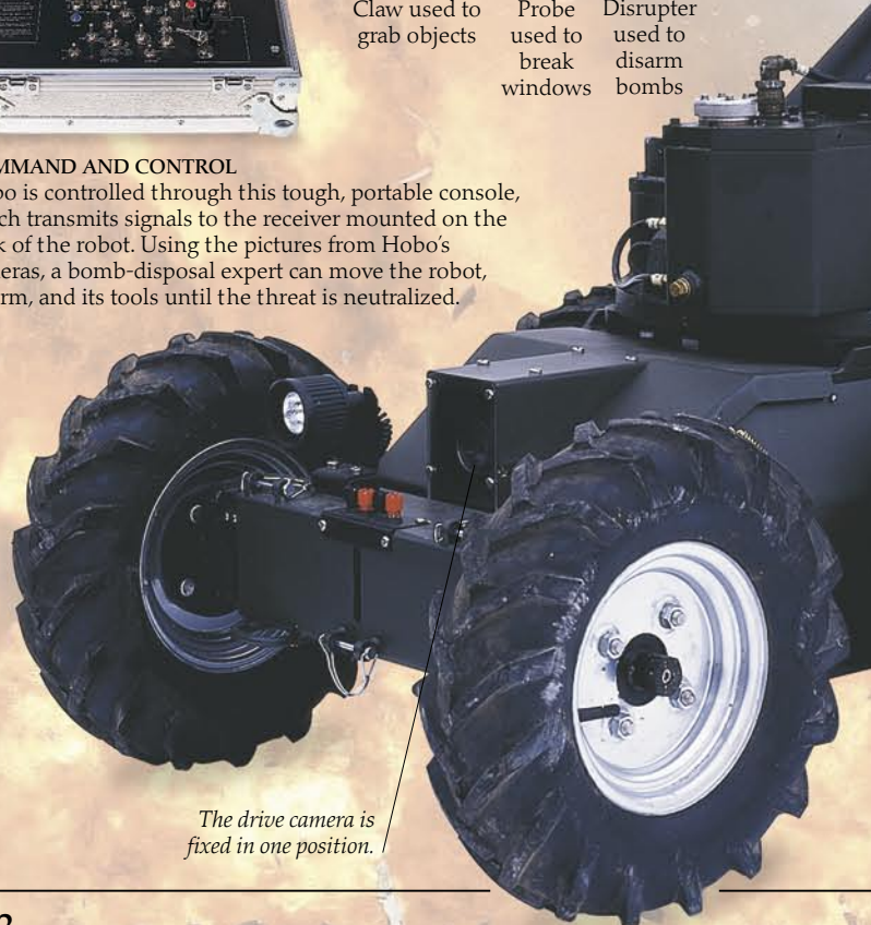
Hobo's low center of gravity enables it to balance at steep angles.
