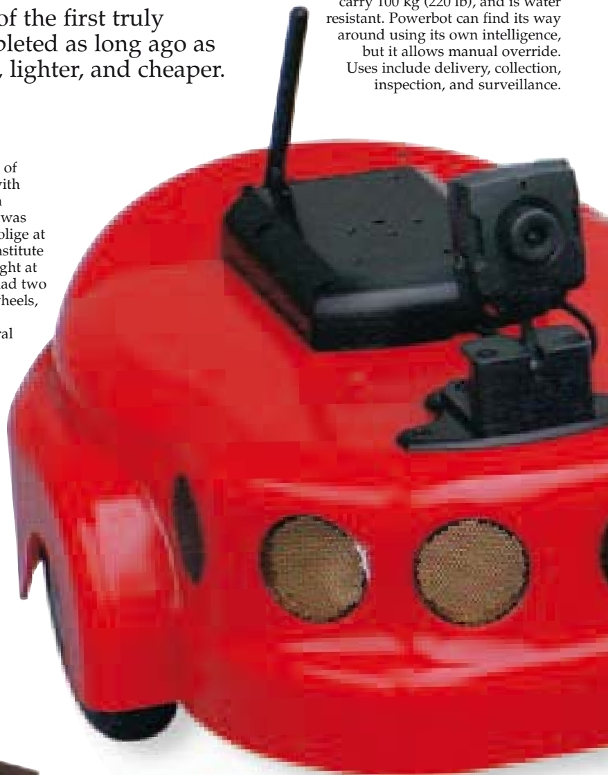
TEAM PLAYER Designed for home-help and education, as well as professional research, Amigobot is based on Pioneer. Teachers like this robot's sturdy reliability and its versatile programming options. It is also designed to work in teams (pp. 56-57) with other Amigobots and can be adapted to play football.
