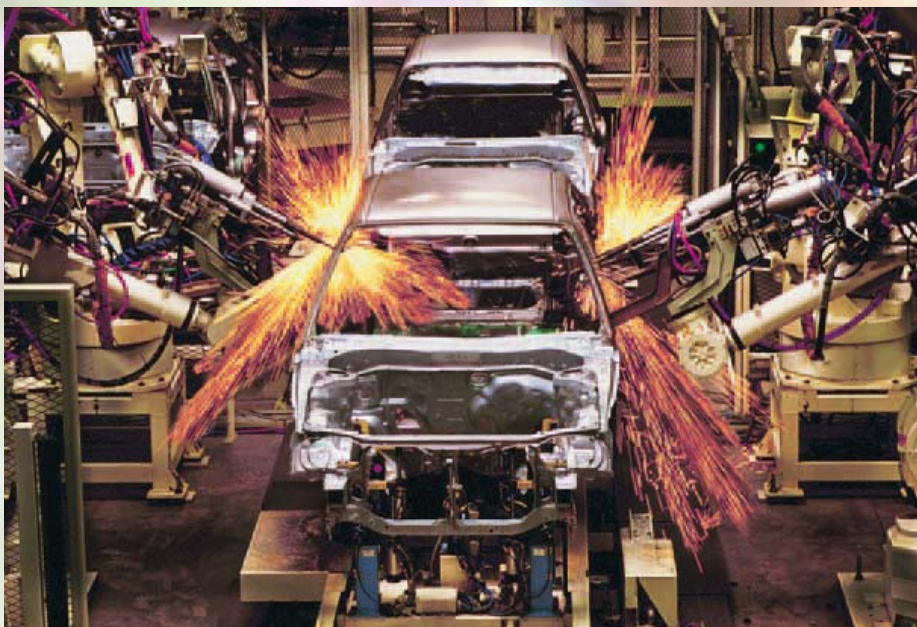
Robot arms welding on a car production line
