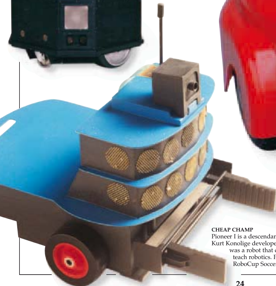
READY-MADE FAMILY Flakey was one of a line of mobile robots starting with Shakey and ending with today's ready-mades. It was developed by Kurt Konolige at the Stanford Research Institute in the USA. A heavyweight at 140 kg (300 lb), Flakey had two independently driven wheels, 12 sonar rangefinders, a video camera, and several on-board computers.
