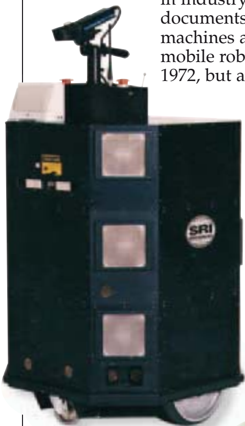
READY-MADE FAMILY Flakey was one of a line of mobile robots starting with Shakey and ending with today's ready-mades. It was developed by Kurt Konolige at the Stanford Research Institute in the USA. A heavyweight at 140 kg (300 lb), Flakey had two independently driven wheels, 12 sonar rangefinders, a video camera, and several on-board computers.
