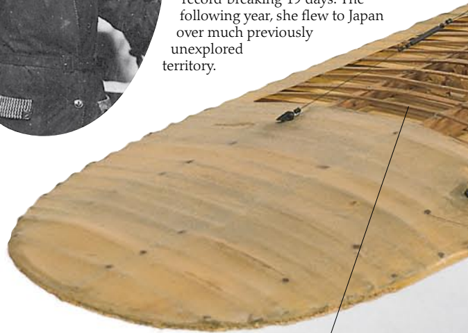
Wooden spars to shape and strengthen wing
