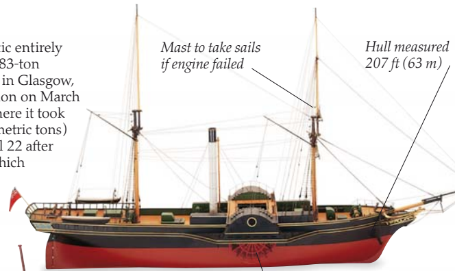
Paddle wheels driven by steam engine
