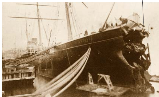
33-ft (10-m) gaping hole in Arizona's crumpled bow
