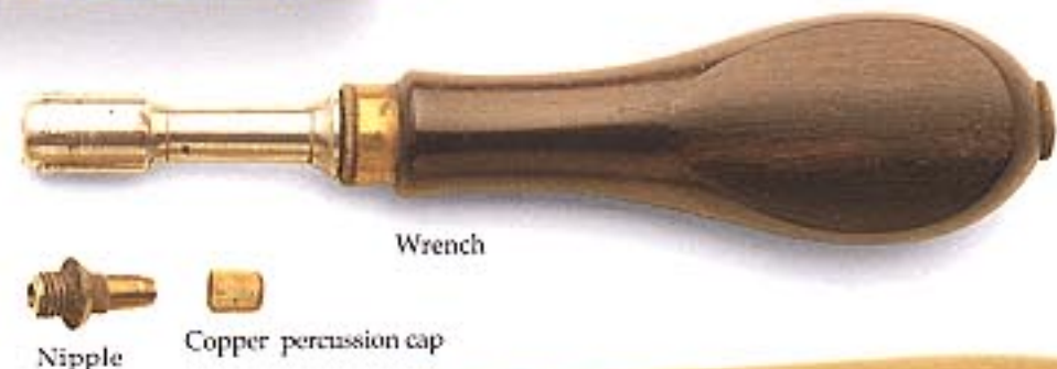
NIPPLE AND WRENCH The nipples, the most vital part of a percussion weapon, were removed by means of the wrench for cleaning. A nipple screwed into the revolver to link the flash of the percussion cap to the propellant.
