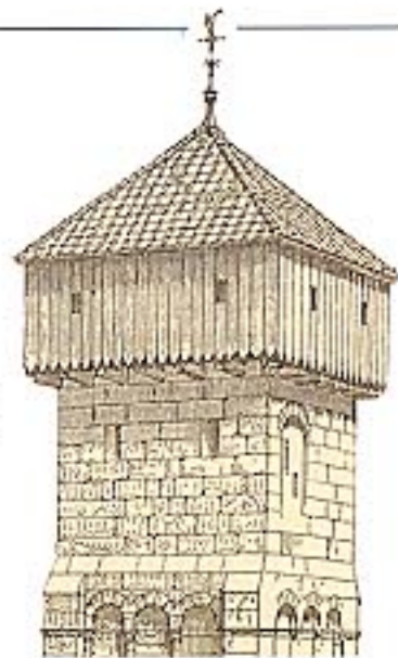
HOARDINGS Removable wooden hoardings were supported on beams pushed into holes called putlog holes below the battlements.
