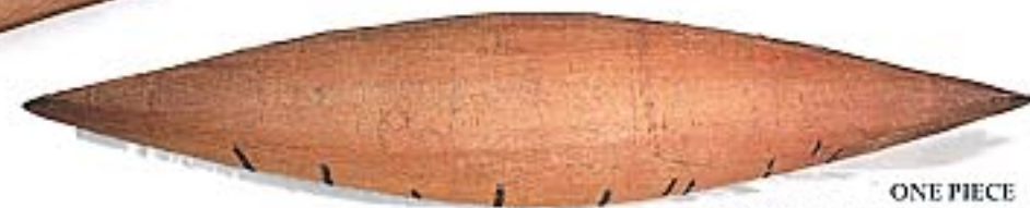
ONE PIECE A bottom view shows that this Algonquin canoe is made from a single piece of bark. Larger canoes are made by sewing on extra sheets.
