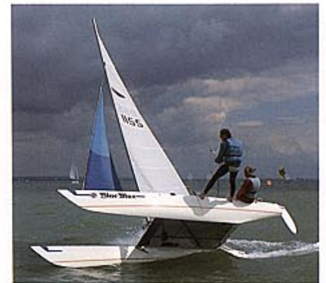
DARTING ABOUT The dart is a catamaran, a twin hulled boat (p. 60). Because these boats are so wide, they can carry a lot of sail, so they are very fast and make for exciting sailing. The dart has no centreboard or boom, which keeps the cost down.
