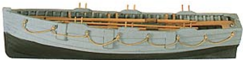
FLOATING TENDER There is no clear distinction between a boat and a ship, but you can say a boat can be put on a ship, but a ship can't be put on a boat! This is a "tender", a small boat used to ferry people and goods between a ship (or a bigger boat) and the shore. It is made of wooden planks, though boats can be made of anything that can be formed into a hollow shell.
