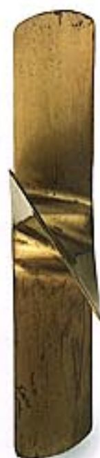
BLADE EDGES The blades of a propeller (in this case a common screw) are helices - like sections of a spiral.
