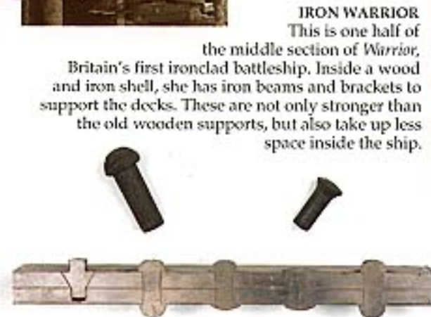
METAL PEGS These are some of the types of rivets used in shipbuilding to fasten overlapping iron or steel plates together.
