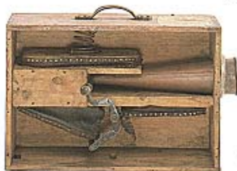
BELLOWING OUT Fog is a great danger at sea, for it obscures rocks, lighthouses, and other ships from view. The handle on this portable fog horn pumps a set of bellows to produce a wailing sound, which alerts other vessels to the ship's presence.
