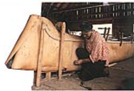
FINISHING TOUCHES Unlike skin boats, bark boats are made shell first. This canoe shell is nearly finished. The separate pieces of bark are in place and are being sewn together with spruce roots. When this is done, all the sewing holes will be sealed with spruce gum. Then the ribs will be added and the canoe will be ready to float.
