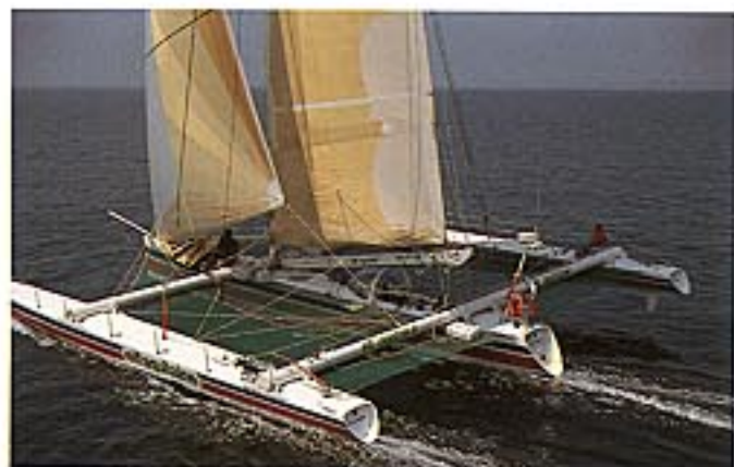
THREE HULLS The Pacific islanders developed multi-hulls – boats with two or more hulls – many centuries ago. They have only been used in the West for offshore racing since the 1960s. This is Elf Aquitaine III , a French high-speed trimaran – a boat with three hulls. It is very stable and cannot roll over, though in the wrong conditions it may turn stern over bow.
