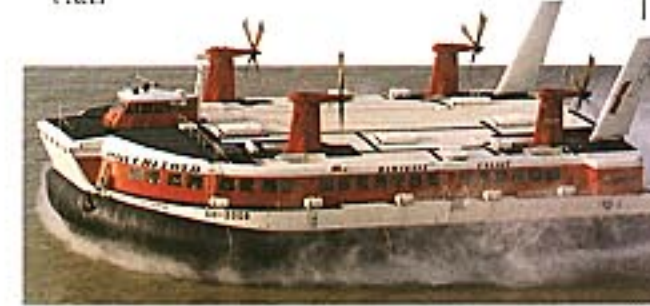
WHAT IS NOT A BOAT? Though it travels across water, a hovercraft is not a boat or a raft because it does not come into contact with the water. It sits on a cushion of air about 20 cm (8 in) above the surface with its whirring propellers pushing air, not water.
