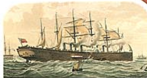
BEST OF BOTH WHIRLS Launched in 1858, the Great Eastern (p. 47) was six times bigger than any ship yet made. She had both paddle wheels for shallow water and a screw propeller for speed in the open ocean.
