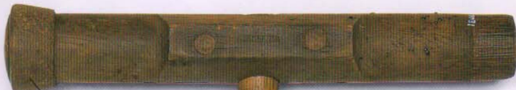
Mallet for striking the irons
