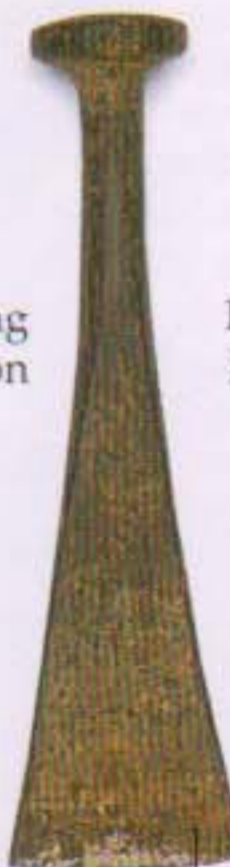
Narrow blade for driving in new oakum
