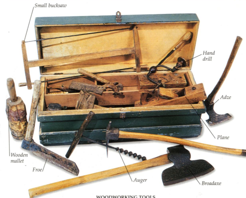
WOODWORKING TOOLS Carefully maintained tools were brought West in stout chests. This tool box, taken on the Oregon Trail, has a broadaxe and adze for shaping logs, augers for boring holes, and a variety of small hand tools for finishing wood and making furniture.
