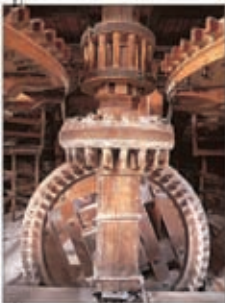
The sails of this traditional windmill transmit power via mechanical gears. A rotating cog operates an adjacent wheel to drive the water pump.
