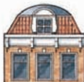
19th-century cornice with mansard roof
