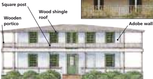
Larkin House (1837), built by Thomas Larkin, was the first Monterey-style house, with its two stories of adobe brick.
