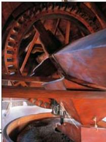
The molino's grinding mechanism is simple: rotating sails turn a vast cogwheel, which connects directly with the grind wheel.
