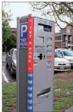
Parking meter operated with coins, credit card or by text message
