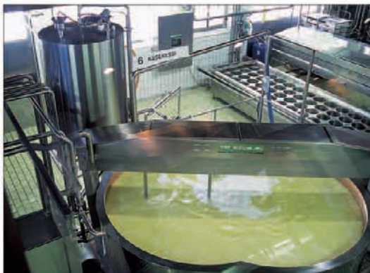
Heating and stirring milk in a vat in a modern cheese factory
