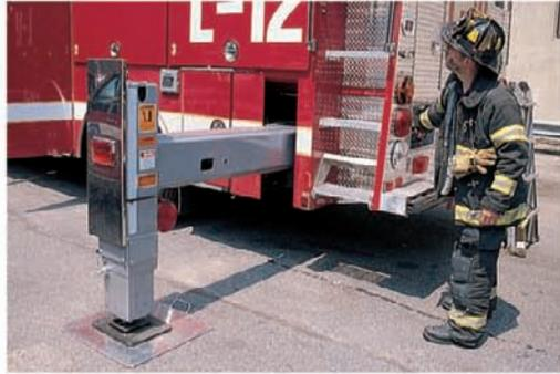
Outriggers are like legs. They keep the truck steady as the ladder is raised. The ladder goes up like a telescope to the top of the house.
