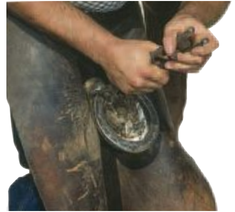
1 REMOVE OLD SHOE The horse stands patiently while the farrier carefully levers off the worn old shoe.
