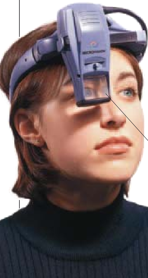
A laser projector produces the images.
