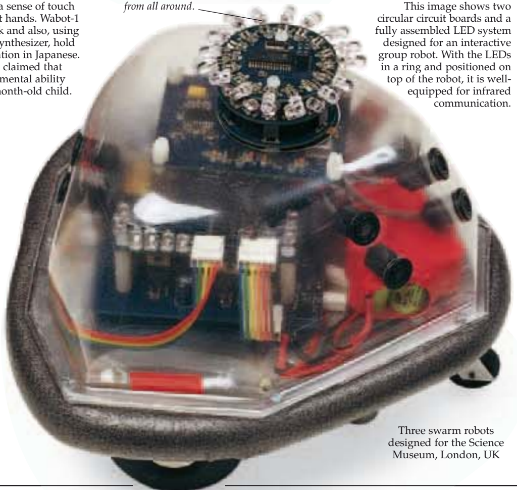
This LED system is fully assembled and ready to be put to use.
