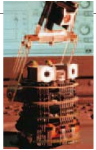
The cameras, which look like eyes on stalks, can tilt to get a panoramic view of the robot's surroundings.
