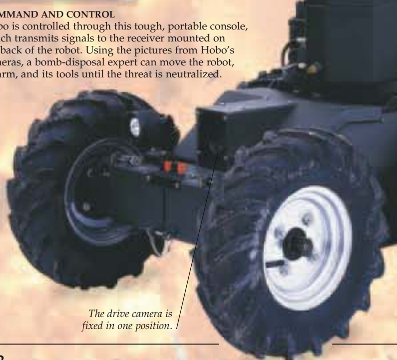
Hobo's low centre of gravity enables it to balance at steep angles.
