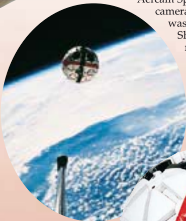
The camera is protected from collisions with other equipment by the cushioned surface.
