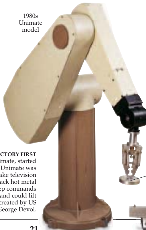
Unimate can be programmed to position parts with great accuracy.
