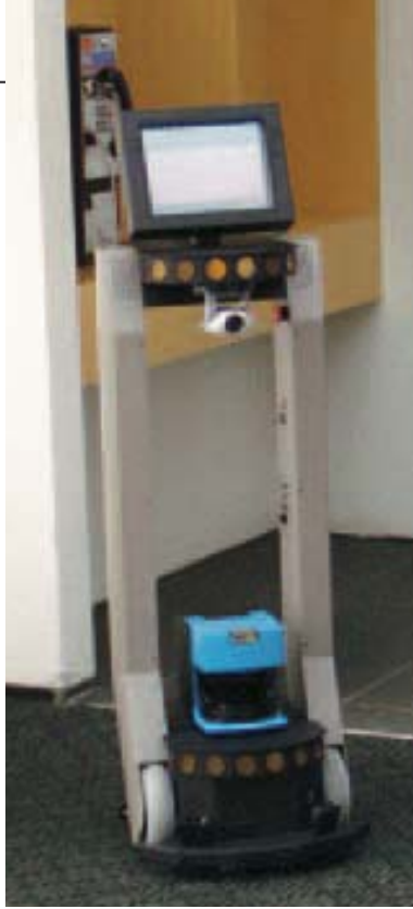
A colour camera takes snapshots of what the robot sees.
