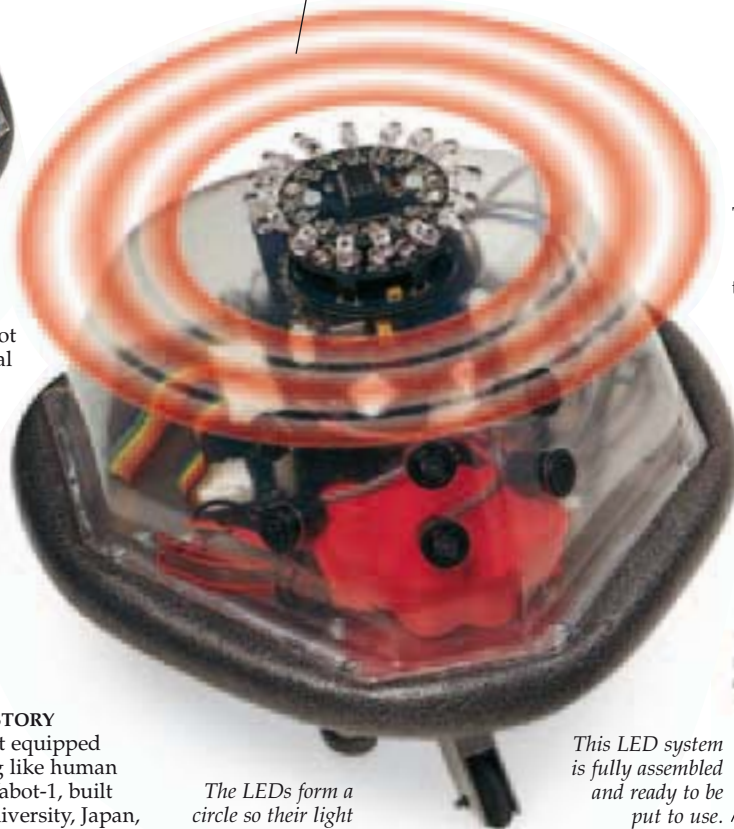
The rubbery bumper contains bump sensors.
