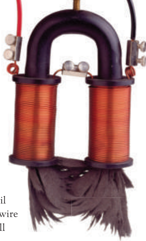
An electromagnet can lift iron filings.
