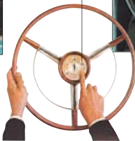
TELETOUCH Teletouch button sent a signal to the car's "precision brain".
