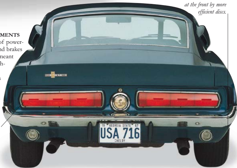
LIGHTS For the Shelby, the Mustang's rear lights were replaced with the '65 T-Bird's sequential lights.
