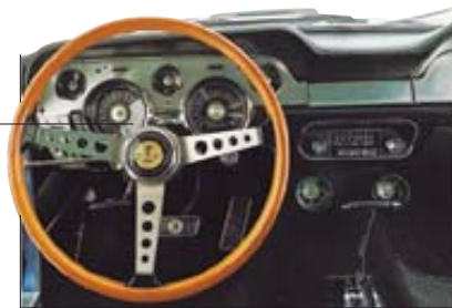
INTERIOR Stewart-Warner oil and amp gauges and a tachometer were standard fittings. Two interior colours were available – parchment and black. Interior decor was brushed aluminium with moulded door panels and courtesy lamps.
