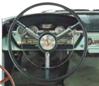
TELETOUCH Teletouch button sent a signal to the car's "precision brain".
