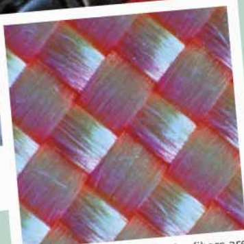
Despite their strength, Kevlar fibers are flexible enough to be woven into fabric. They are also used in ropes.
