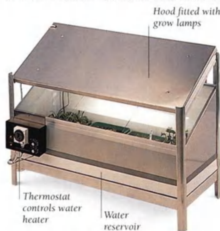
FOG PROPAGATION UNIT This unit pumps fresh air through a water reservoir, creating a warm "fog" around the propagated material without wetting the leaves. Vapor condenses on the sides and runs back into the reservoir.
