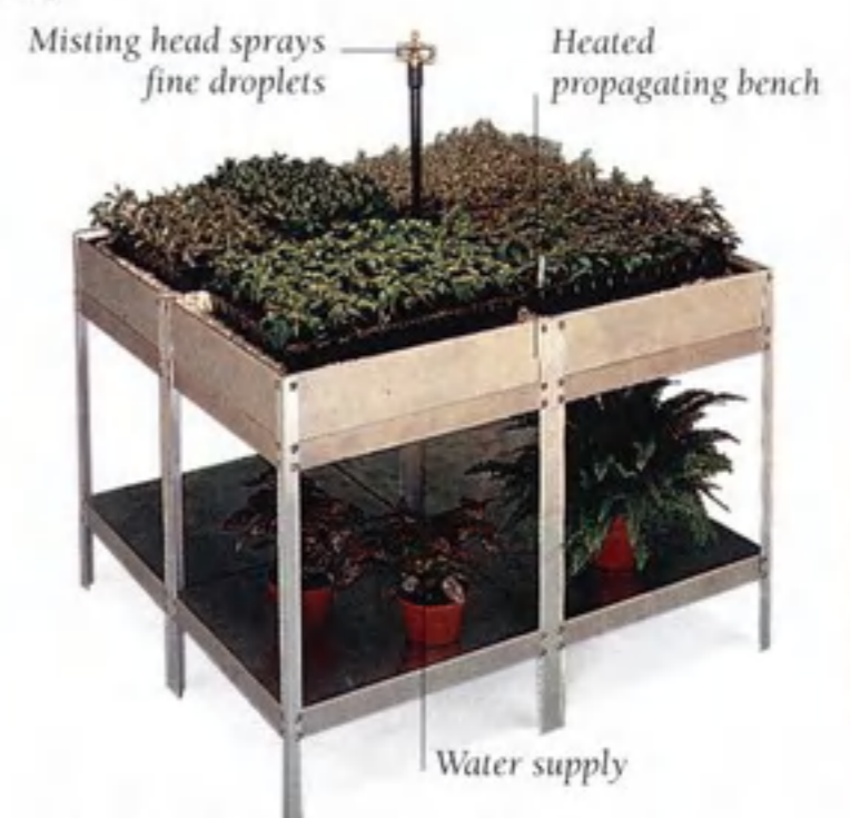
MIST PROPAGATION UNIT The misting head automatically delivers an intermittent spray of fine droplets over the propagated plants. The heated bench aids rooting, while the mist cools the topgrowth and prevents moisture loss.
