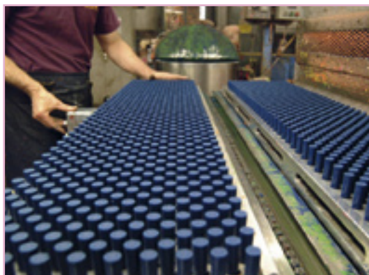
4 Hardening It takes a few minutes for the mixture to cool and harden into crayons. The new crayons are lifted out of the moulds.
