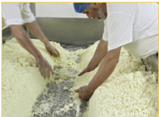
5 Drain and cool The whey is drained off and the curd, which will become the cheese, is transferred into a slightly sloping cooling tray where the moisture drains away.
