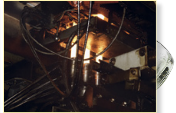
5 Cutting gobs The molten glass flows from the furnace along channels. Then it is chopped into lengths, called gobs, each exactly the right size to make one bottle.
