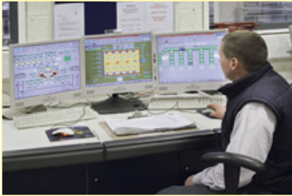
3 Computer control The factory is controlled by computers. These manage the furnace temperatures, and the speed bottles are made and moved through the factory.
