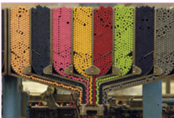
8 The sorting machine Workers choose the colours they need for a particular selection box, and tip them into a collating machine.
