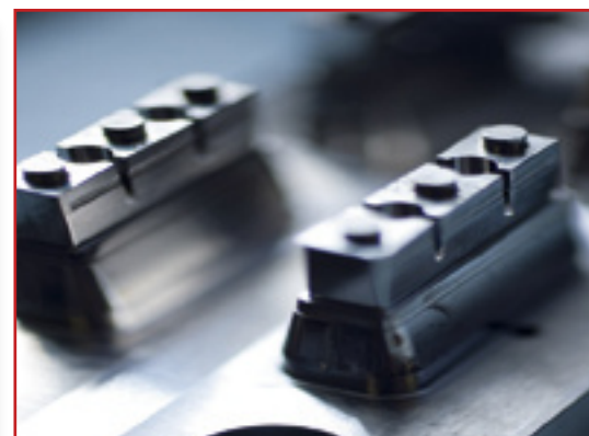
5 Moulding bricks The melted granules are poured into brick-shaped moulds. Then moulds like the ones shown here are pushed into the soft plastic to make the insides of the bricks.
