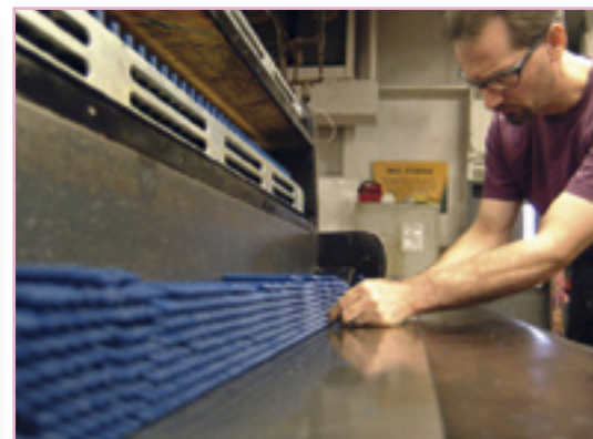
5 Inspection time! All the crayons are checked for quality. Any that have holes or bits missing are remelted and remade.
