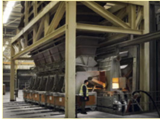
4 Mix and melt The ingredients are mixed together, then tipped into a huge furnace. Heated to 1500°C (2732°F), the mix melts to a liquid. This is molten glass. It is so hot that it glows white.
