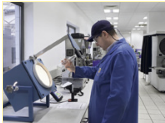
10 Quality checks Bottles are regularly checked and tested for quality. They have to be perfect. Any that don't make the grade are sent back to the furnace for recycling.
