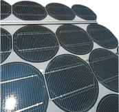
SOLAR POWER Nearly all our energy comes from the sun. Solar cells let us tap this energy directly, using lightsensitive crystals to convert sunshine into electricity. Solar power is only practical in places with plenty of sunshine.
