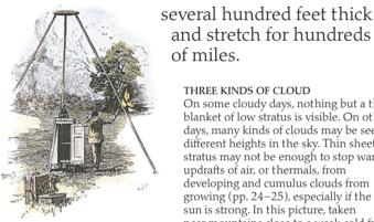
MEASURING CLOUD HEIGHT The Victorians calculated the height of clouds by using cameras and giant tripods, but meteorologists nowadays use laser beams pointed at the base of the cloud to judge its height. Cloud cover, however, is worked out visually, by estimating roughly what proportion of the sky is obscured by the cloud directly overhead - usually in tenths or eighths.
