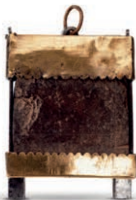
LODESTONE The earliest type of magnetic compass.
