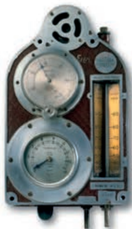
EARLY AIRCRAFT INSTRUMENT PANEL Showed aircraft's height and speed.
