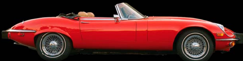
The 1961 Jaguar E-Type's shape was the work of an airplane designer. It's very sleek, but the shape of the back creates lift, which can ruin grip.
