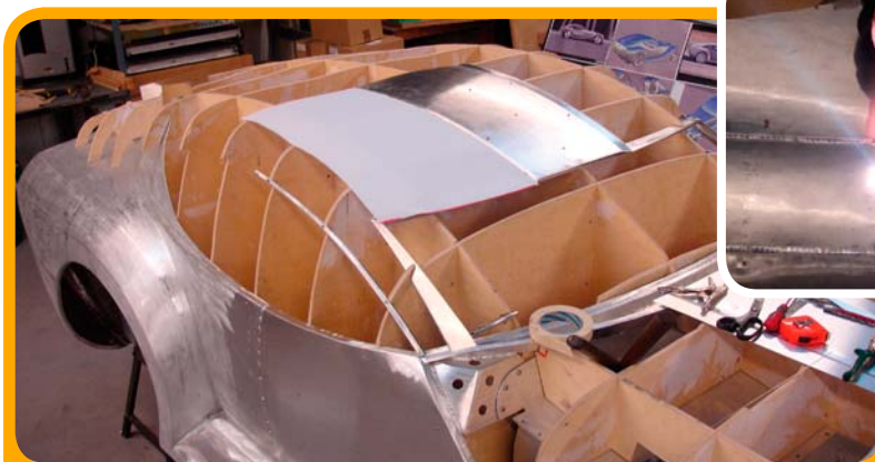
To make the outer skin, the computer model is used to make an “egg carton” out of wood. Aluminum is then rolled and cut to fit.
