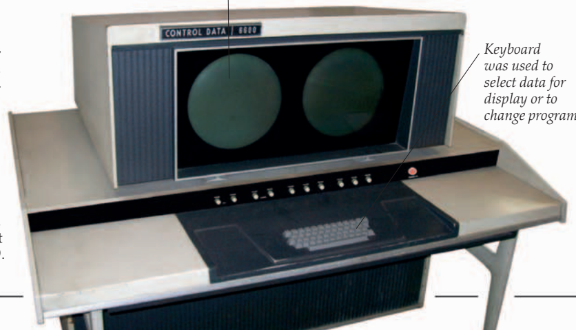
Display screen for text and simple graphics
