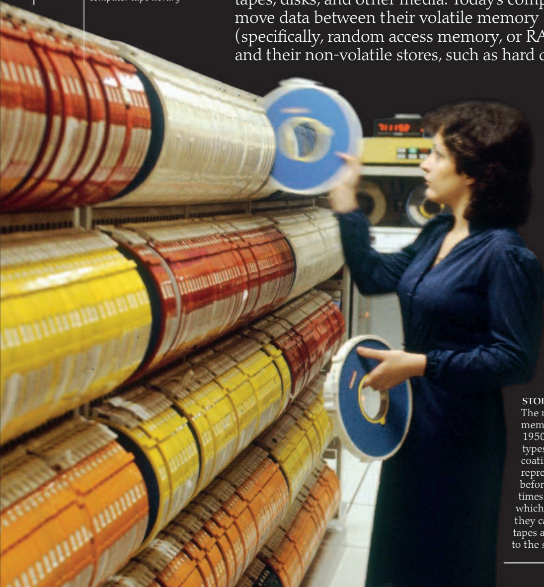
Magnetic data storage tapes in a rack, in a computer tape library
