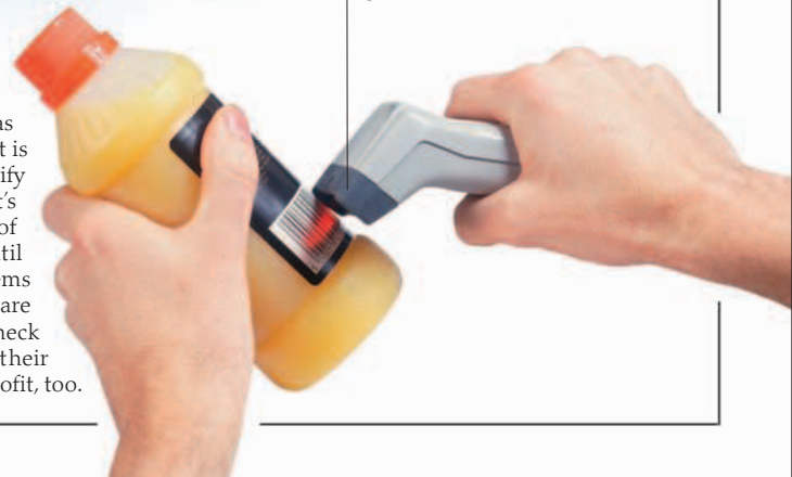
Bar code reader uses a laser to scan bar code data, which is then matched against a database
