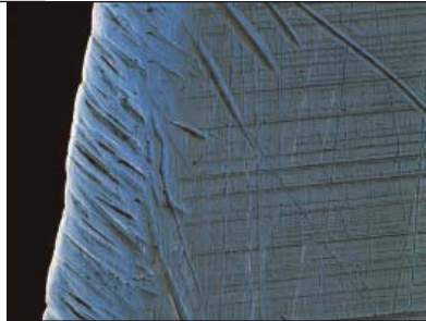
Worn edge of a steel razor blade
