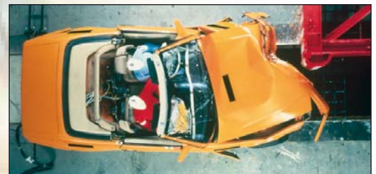
Aerial view of a car during a crash test
