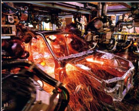
Robot worker welding a car
