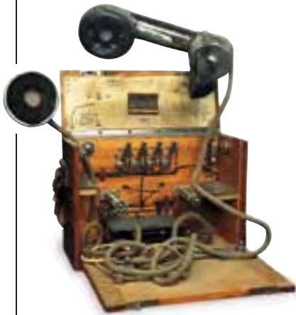
FIELD TELEPHONE Telephones were the main communication method between the front line and headquarters. They relayed voice and Morse code messages.
