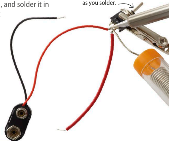
Hold the switch in the third-hand tool to keep it in place as you solder.
