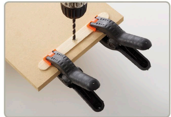
Use scrap wood underneath your item so you don't drill into your work surface.
